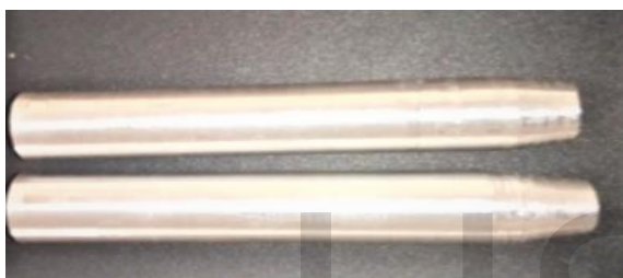
Fig. 2. Samples machined for ECAP processing
